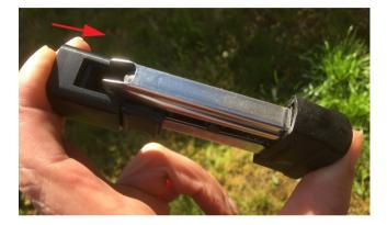
Step 2: Insert the cartridge on the magazine.
